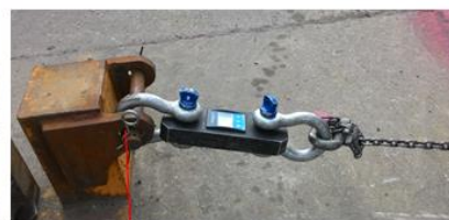
Pry post connected with Load Cell, D shackle & chain
