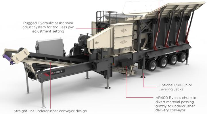
Straight-line undercrusher conveyor design reduces slippage; mechanical raise/lower system lowers tail section for maximum undercrusher clearance, raises tail section for ease of clean-up, unit locks into raised position for travel
