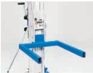
**STANDARD FORKS** accommodate a variety of general loads. Get an additional 21 in (53 cm) of lift by turning over and re-pinning the forks.
