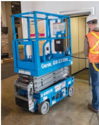
This lightweight scissor lift is able to access jobsites previously off limits to heavier slab scissors and vertical mast lifts in the industry due to passenger elevator capacity limitations
