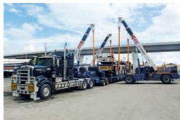
Terex Pick & Carry cranes live up to their name with the strength and easy operation to pick up heavy loads and the steering flexibility to move in tight spaces. Their high road speeds get them to the jobsite quickly, and because the articulated frame needs no outriggers, you can get set up and working almost immediately.
