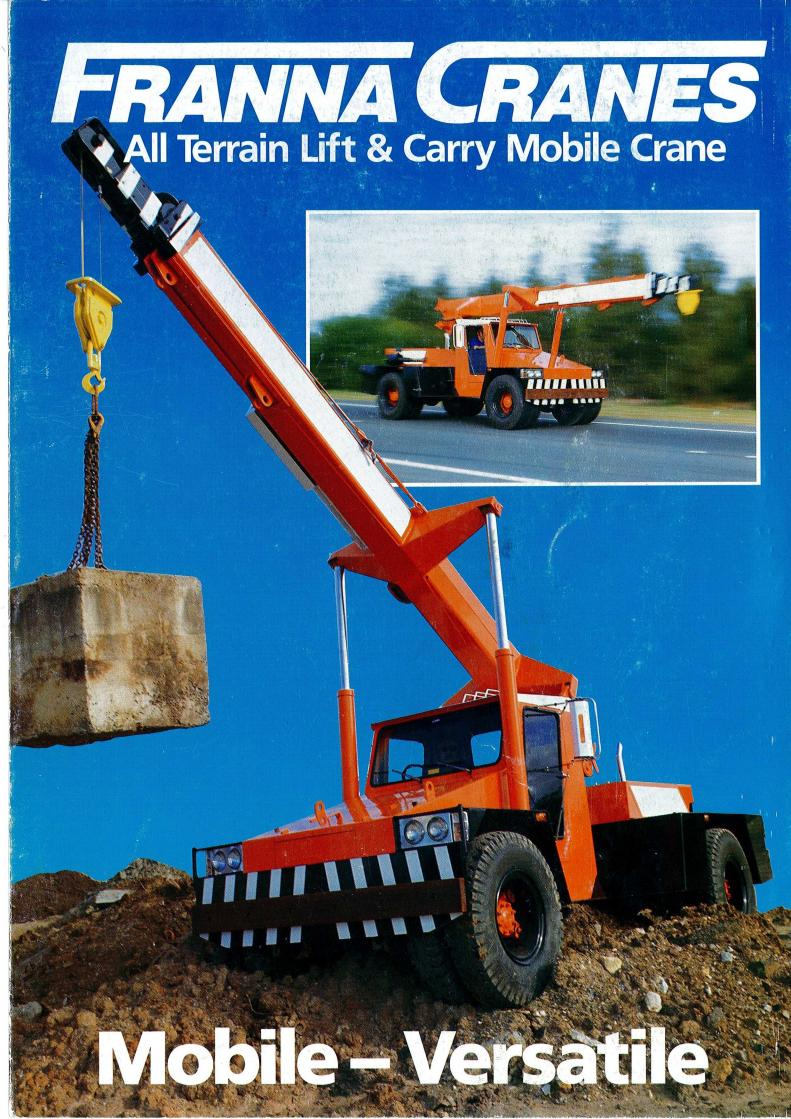
his is the first Allterrain Articulated Lift and Carry Mobile Crane, fully designed and built in Australia. It is ideal for general hire and site work.
