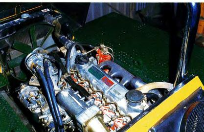
Total engine cover is hinged to open rearward for maximum access to 163 HP diesel engine and service points. Upswept exhaust for minimum noise levels.
