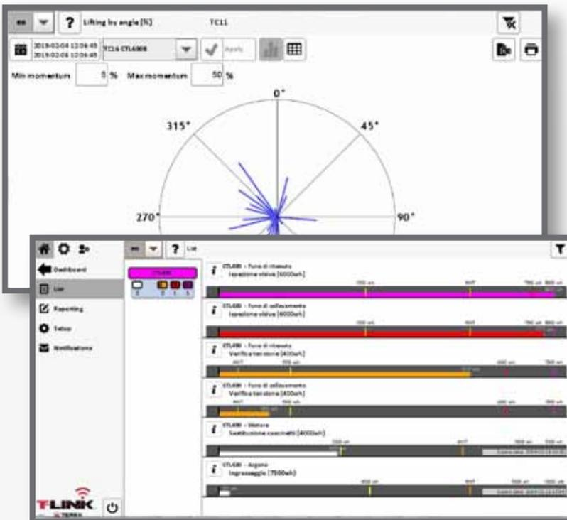
**T-Link** has 11 analytics templates and if not enough, you can use T-Link's configurable analytics engine to create your own combinations of 35 parameters. You can monitor parts wear and under which conditions the crane has been operating. Moreover, you can predict maintenance needs. Data can be visualized as charts or tables, printed or downloaded. If you run a rental business, T-Link analytics allows you to bill operational time and stand by time differently.
