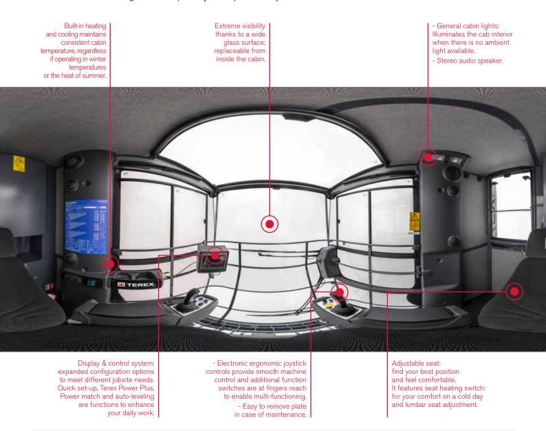
Explore a 360° view of the new Terex tower crane cabin available on select models at info.terex.com/tower-cabin
