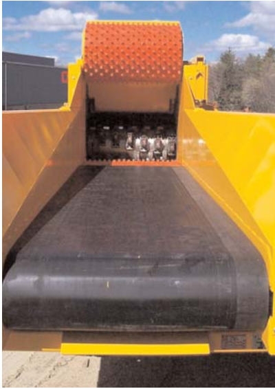
Large feed opening to allow easy processing of whole trees and provide for easy maintenance.
