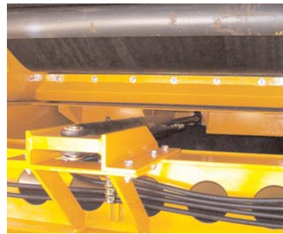
Hydraulically activated regrind pan that prevents pre-screening of material allowing very fine material to be produced.
