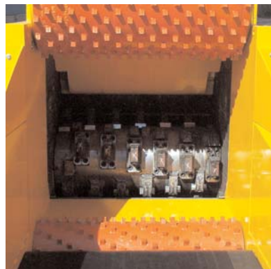
Large feed opening to allow easy processing of whole trees and provide for easy maintenance.
