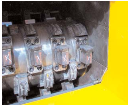
Heavy-duty internal top feed roller drive
