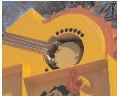
Heavy-duty internal top feed roller drive
