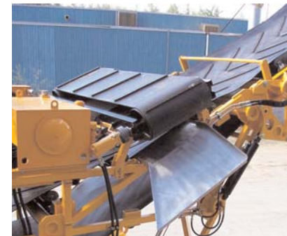
Optional Overband Magnet and Magnetic Head Pulley with discharge chutes for maximum metal recovery. Overband Magnet fits under folded conveyor for hassle free transport.
