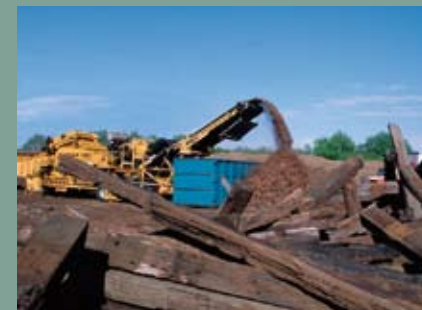
Railroad ties to hog fuel
