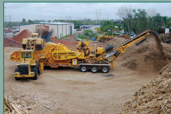
Regrind of Mulch (shows optional overband magnet)
