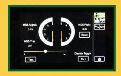
A problem for any industrial grinder has to do with tramp metal entering the hog box and causing significant damage, which leads to downtime. The Metal Detection System™ (MDS) engages within milliseconds whenever the grinder's rotor makes contact with tramp metal. The rotor is monitored by an adjustable electronic sensor to alert
