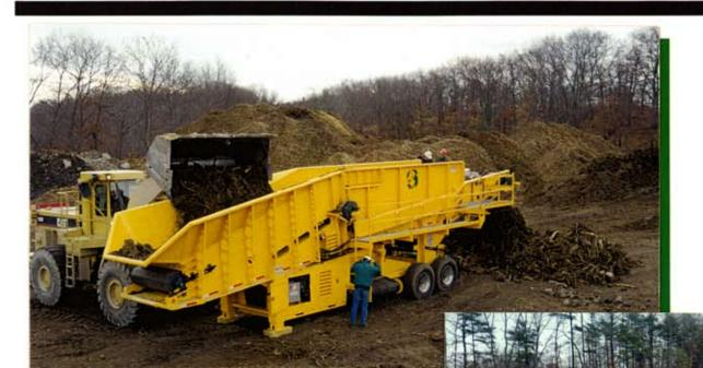
In addition to CBI's line of portable and stationary wood waste processors we offer a portable screener with a screening capacity that easily reaches over 150 tons per hour. The CBI Screener has a built-in picking station for up to four people and is designed to screen landclearing debris, yardwaste, log yard debris and heavily contaminated C & D debris with ease, remove metal contaminants and work in tandem with a CBI grinder.
