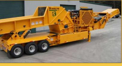
material to be discharged out the back and is designed to be fed by a loader or excavator.
