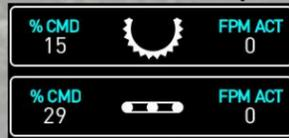
The "% CMD" is the adjustable parameter that changes the feeds speed command output, in percentage, that the feeds will run at. The "FPM ACT" is the actual speed feedback, in feet per minute, that the feeds are running at.
