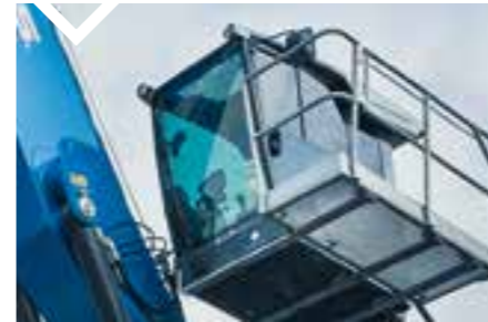
CATWALK WITH HANDRAIL*
