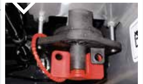
LOG- OUT TAG- OUT BATTERY MASTER SWITCH
