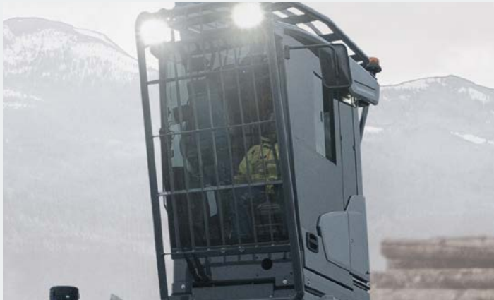
➔ Front and roof guard for timber application
