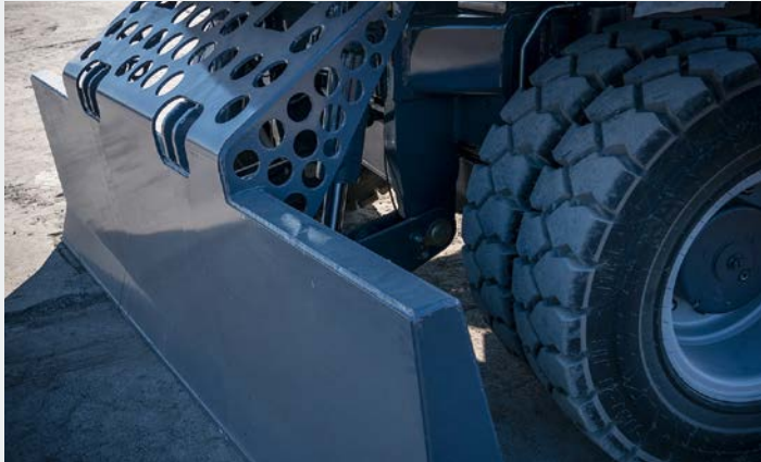
➔ Support blade, integrated cylinder protection
