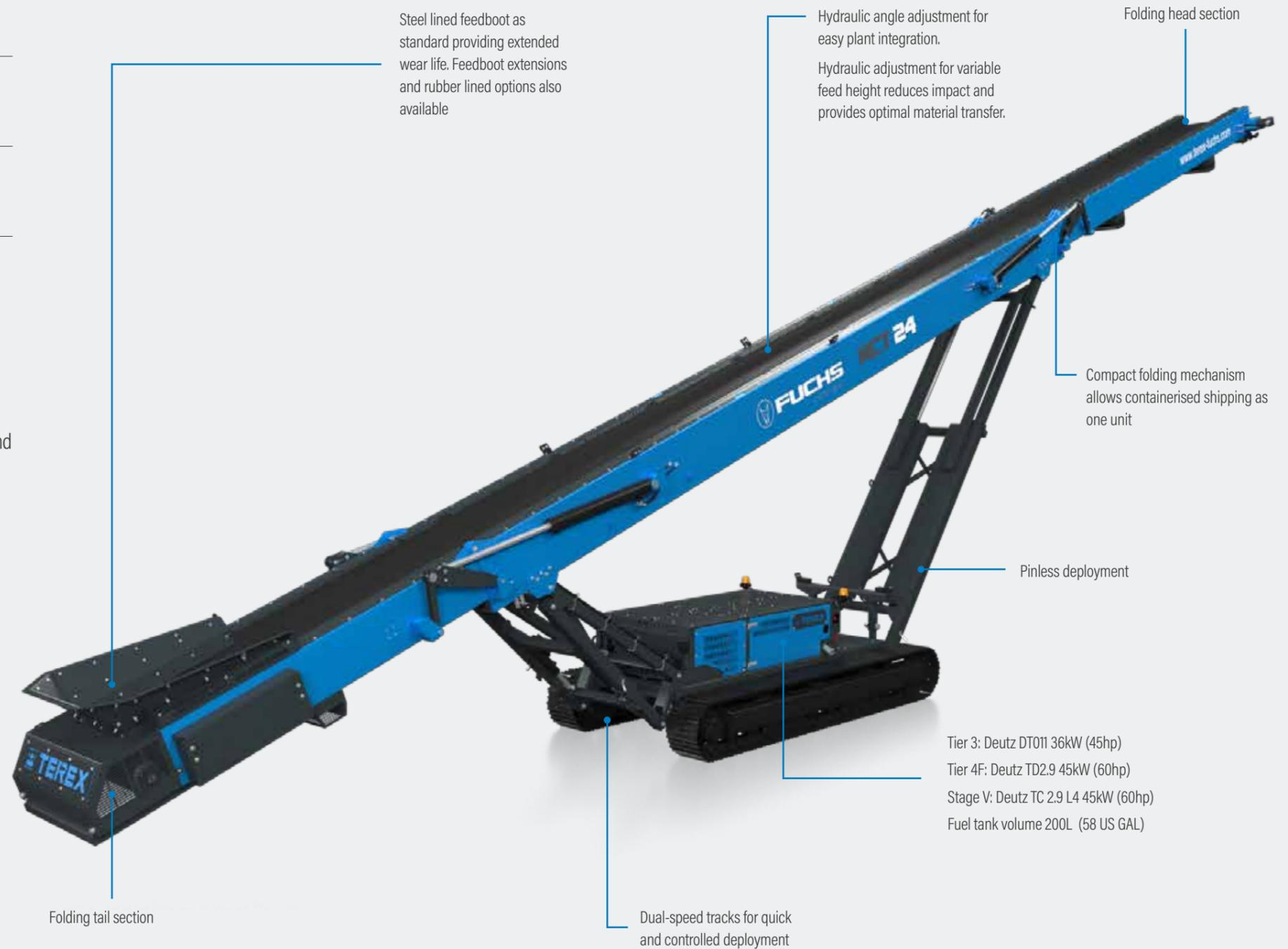
Steel lined feedboot as standard providing extended wear life. Feedboot extensions and rubber lined options also available
