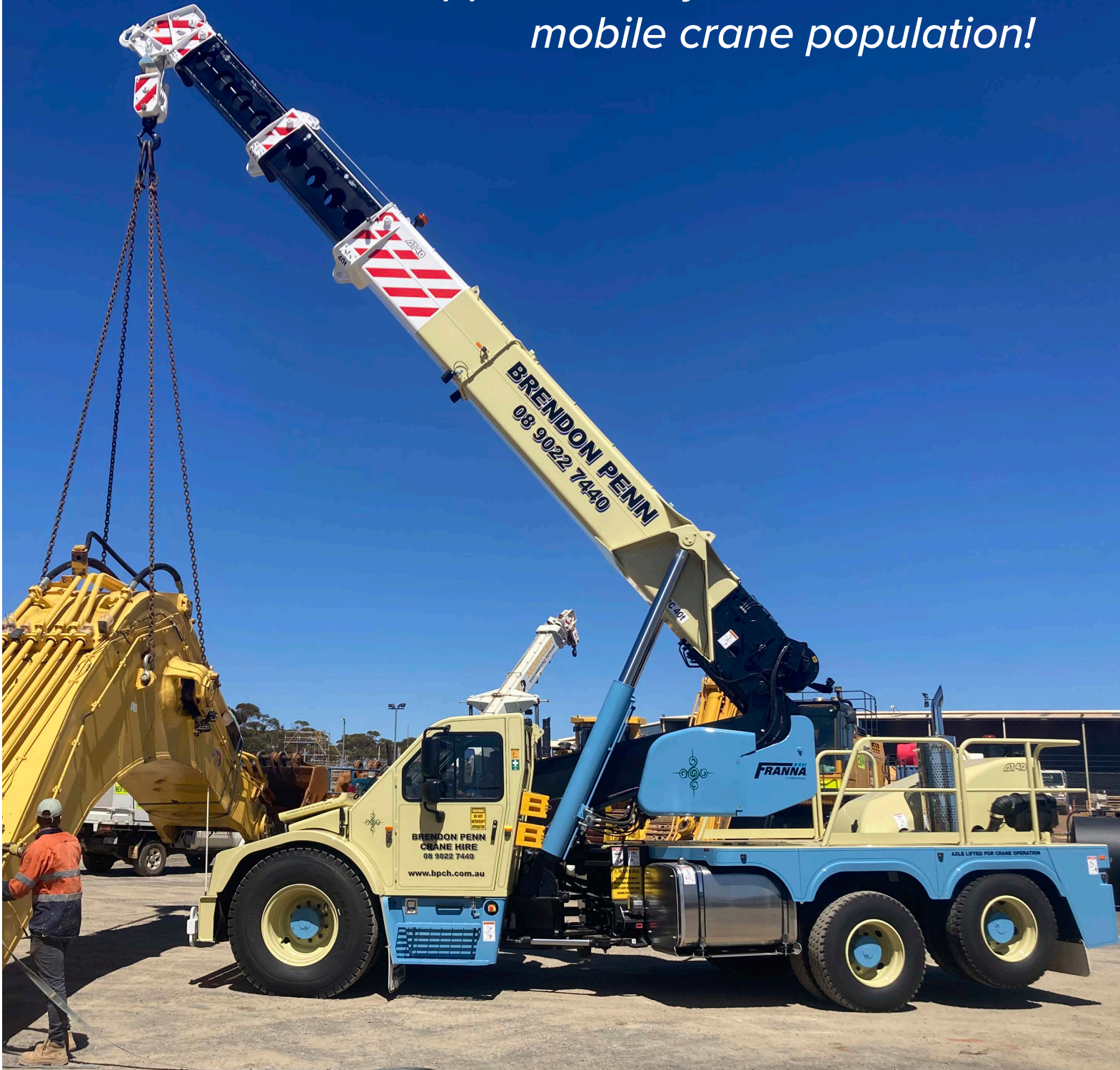
AT 40 lifting 22t boom for a mining excavator / shovel
