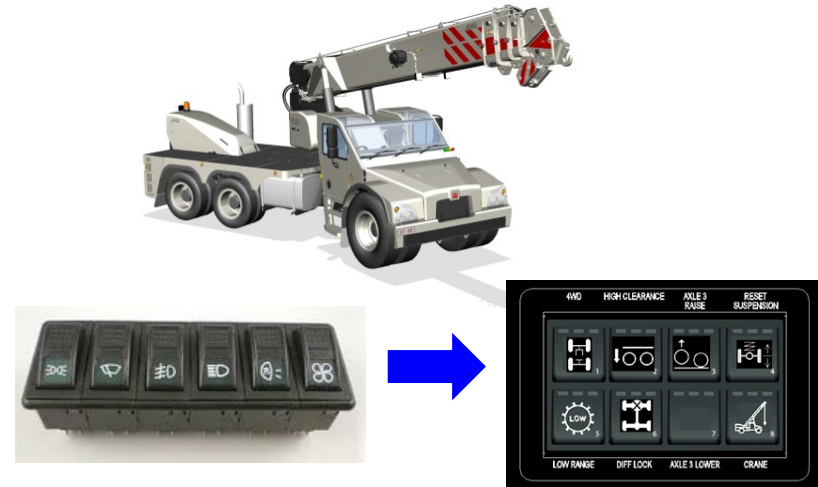
Traditional Rocker switches replaced with CAN keypad
