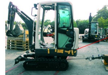
Typical arrangement of machine for Drawbar pull Test.
