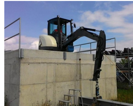
Pry post connected with Load Cell, D shackle & chain
