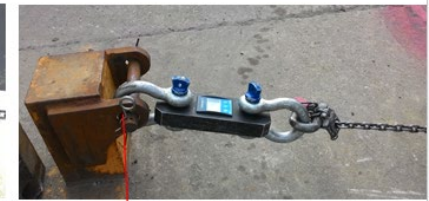
Pry post connected with Load Cell, D shackle & chain
