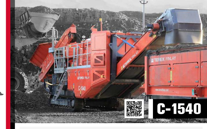
The fuel efficient direct drive Terex Finlay C-1540 cone crusher is the optimum machine for medium sized producers and contract crushing operators.
