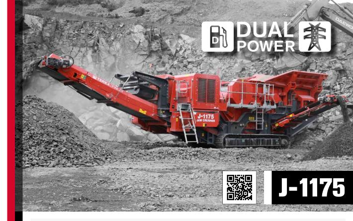
The dual powered Terex Finlay J-1175 jaw crusher offers operators the flexibility to power the plant either by mains electric connection or the onboard genset powerpack configuration. Either power option presents operators with significant power, servicing and maintenance cost savings in direct comparison to a diesel/hydraulic powered plant.
