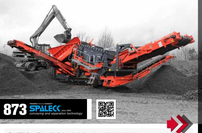
The NEW Terex Finlay 873 Spaleck is ideally suited to working in aggregates, sand and gravel, top soil, construction demolition and recycling applications. This highly versatile machine can be fed either by a tracked mobile crusher, shovel or an excavator.
