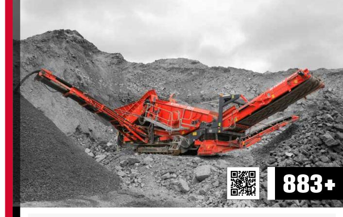
The fourth generation Terex Finlay 883+ has been developed as a high capacity and versatile heavy duty scalper to work in primary and secondary screening applications such as quarry and mining, iron ore, construction demolition waste, sand, gravel, compost, top soil and coal.
