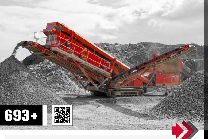
The double deck Terex Finlay 693+ has been designed and developed to fulfill the demands of today's high production producer. The double deck screen configuration provides two full sized 6.1m x 1.53m (20' x 5') screen decks. A high capacity belt feed hopper is available with remote tipping grid or double deck vibrating grid. Impressive features include hydraulic tipping reject grid complete with grouser bars, three on-board hydraulic folding conveyors and low level greasing access points.
