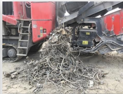
Metal removed by magnet
