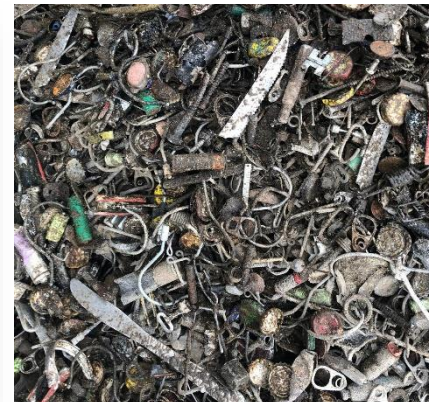
Metal removed by magnet
