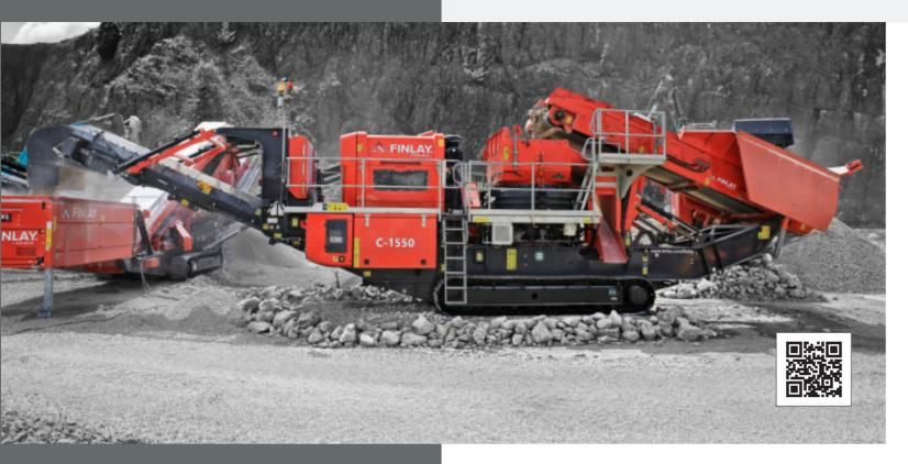
The Finlay<sup>®</sup> C-1550+ cone crusher is designed to be the optimum mobile solution to produce aggregates for road construction and railway ballast as well as for asphalt and concrete fractions.
