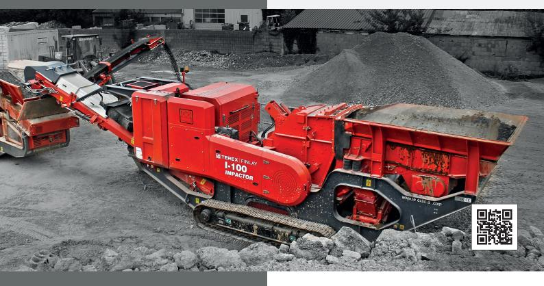
The Finlay® I-100 tracked impact crusher has been specifically designed for quarrying, recycling and demolition applications. The I-100 features a Ø860mm x 830mm (Ø34" x 33") direct drive impact chamber with variable rotor speed. The advanced electronic control system monitors, controls and regulates the speed of VGF with, integrated pre-screen, to maintain a consistent feed of material into the impact chamber while maintaining optimal crushing capacity.
