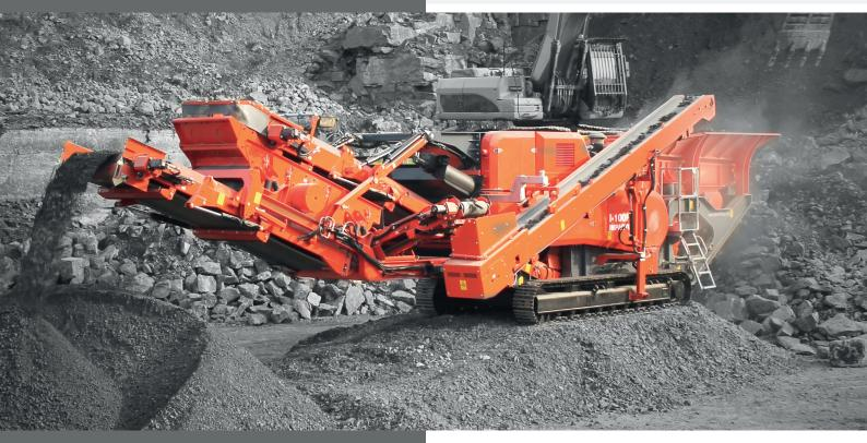
The Finlay® I-100RS direct drive Ø860mm x 860mm (Ø34" x 34") horizontal impact crusher with variable speed gives operators unprecedented levels of fuel efficiency and production in both recycling and quarrying applications. The machine features a  $2.44m \times 1.2m$  (8' x 4') single deck screen for sizing and recirculating oversize material back to the crushing chamber.
