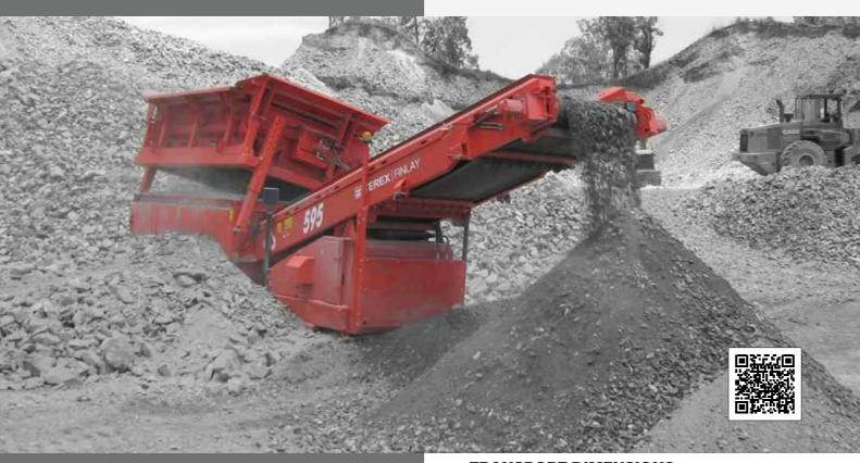
The Finlay® 595 Hydratrak is a self contained, high capacity mobile scalper.
