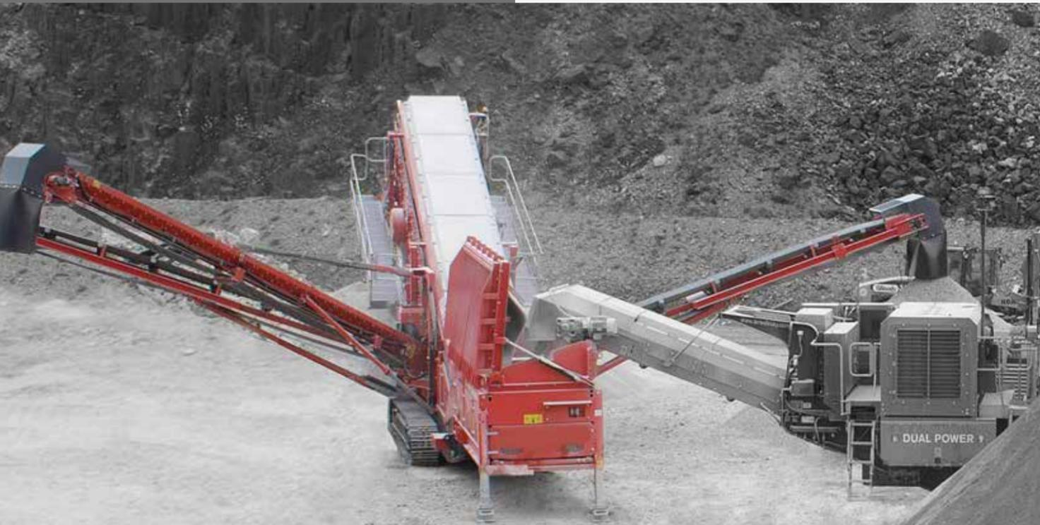
The Finlay® 694+ Hybrid Inclined Screen offers operators the flexibility to power the plant either by an electrical connection or diesel/hydraulic configuration. The plant features a triple deck screen configuration providing three full sized 6.1m x 1.53m (20' x 5') screens.
