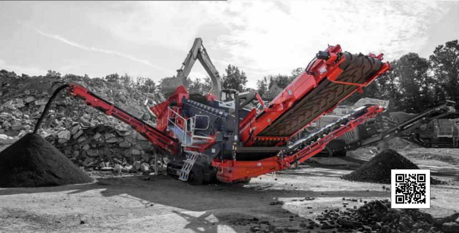
The Finlay® 883+ Spaleck mobile recycling screen is the ultimate in mobile screening and separation technology. At the heart of the screen is the two deck German designed and constructed high performance recycling waste screen with Flip-Flow-Screen Elastica.
