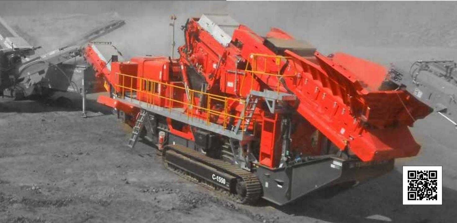
The Finlay® C-1550P incorporates the proven Terex® 1300 cone crusher driven through direct drive.
