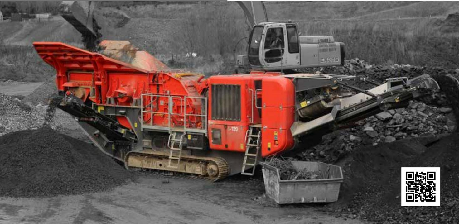
The Finlay® I-120 mobile impact crusher has been designed with improved material flow and enhanced productivity in quarrying, mining, recycling and construction demolition applications.
