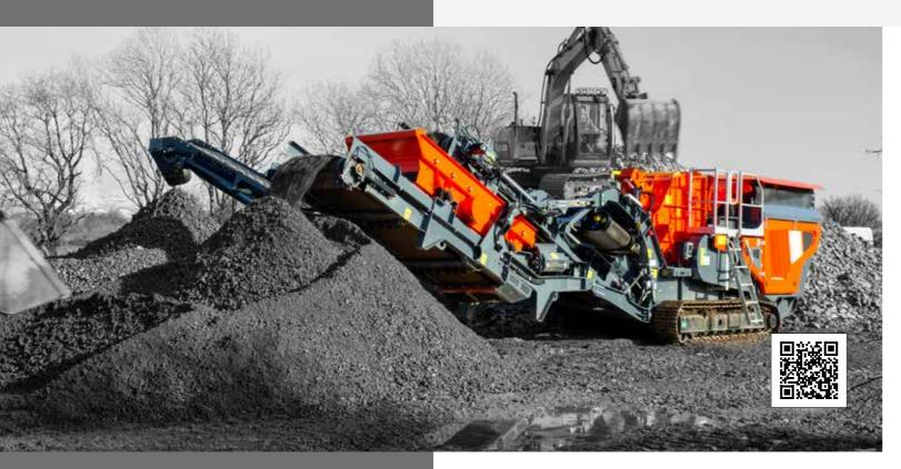
The Finlay® IC-100RS Portable Impact Crusher provides the versatility of a compact crushing and screening plant on one mobile platform for quarrying, construction and demolition debris, reinforced concrete and asphalt recycling applications. The machine features a direct drive ø860mm x 860mm (Ø34" x 34") horizontal impact crusher with variable speed control to give operators high levels of fuel efficiency and productivity.
