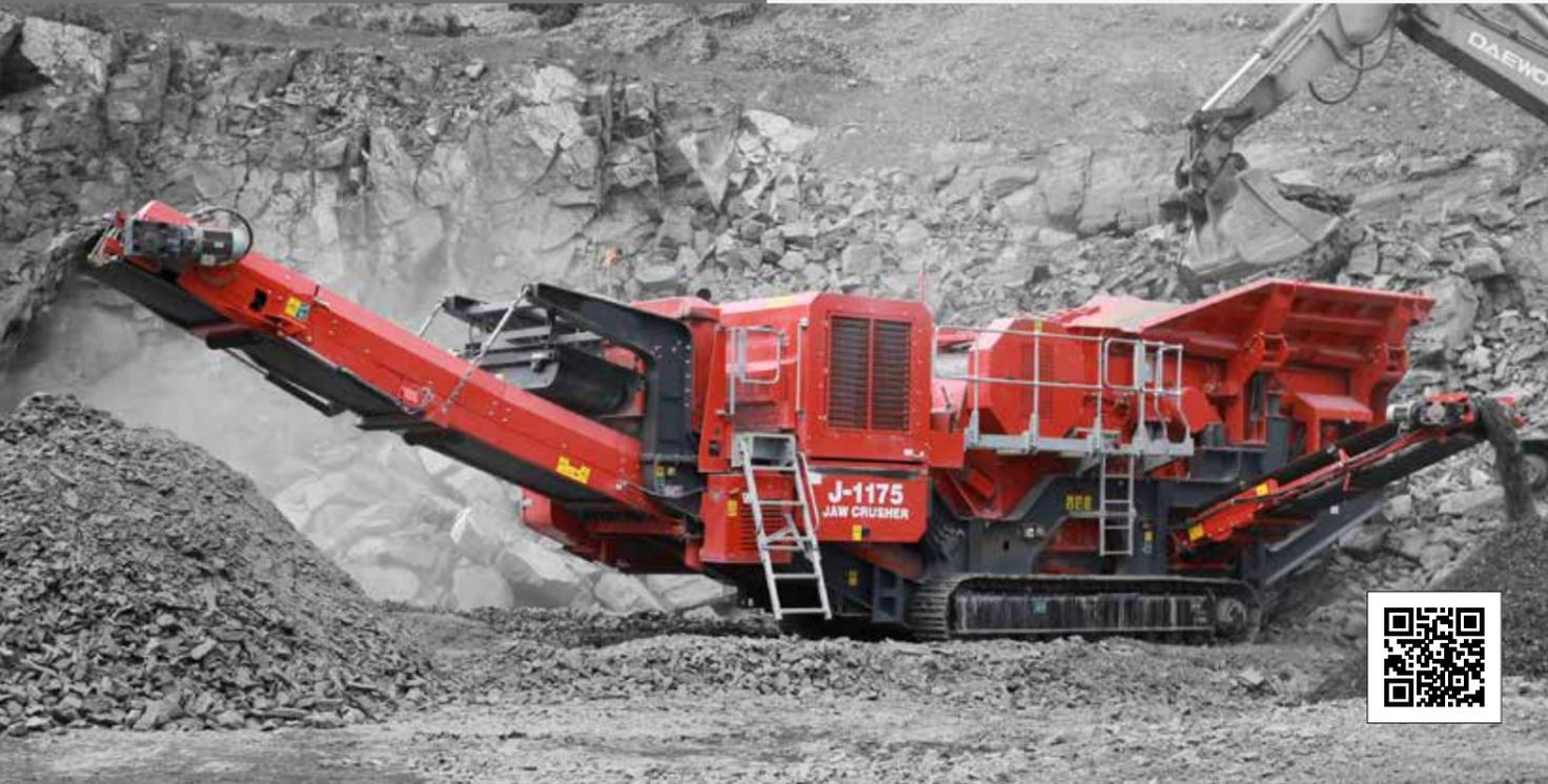
The Finlay® J-1175 hybrid mobile jaw crusher offers operators the flexibility to power the plant either by mains electric connection or the onboard genset powerpack configuration.
