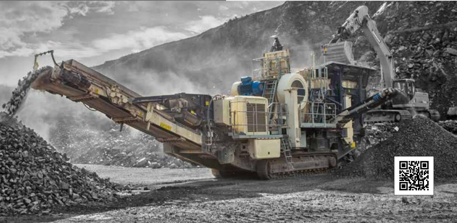
The Finlay® LJ-130 hybrid mobile jaw crusher is the largest mobile jaw crusher in our range and has been developed for large-scale quarry and mining operations. The machine can operate as standalone primary crusher or integrated into a mobile or static crushing and screening plant.
