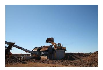
The blended feed material is delivered to the 16x5 screen by a heavy duty inclined feed conveyor fitted with a 1000mm belt. At the head of the conveyor an integrated wash box gives the material an all-important pre-soak to pre-condition before going on to the screen.
