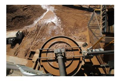
The conical sump is designed to enable regulation of incoming water and solids flowing in varying conditions without the loss of useful fines.
