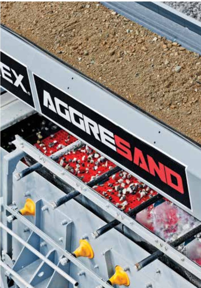
Aggregate Screen Fitted with Isolated Spraybars
