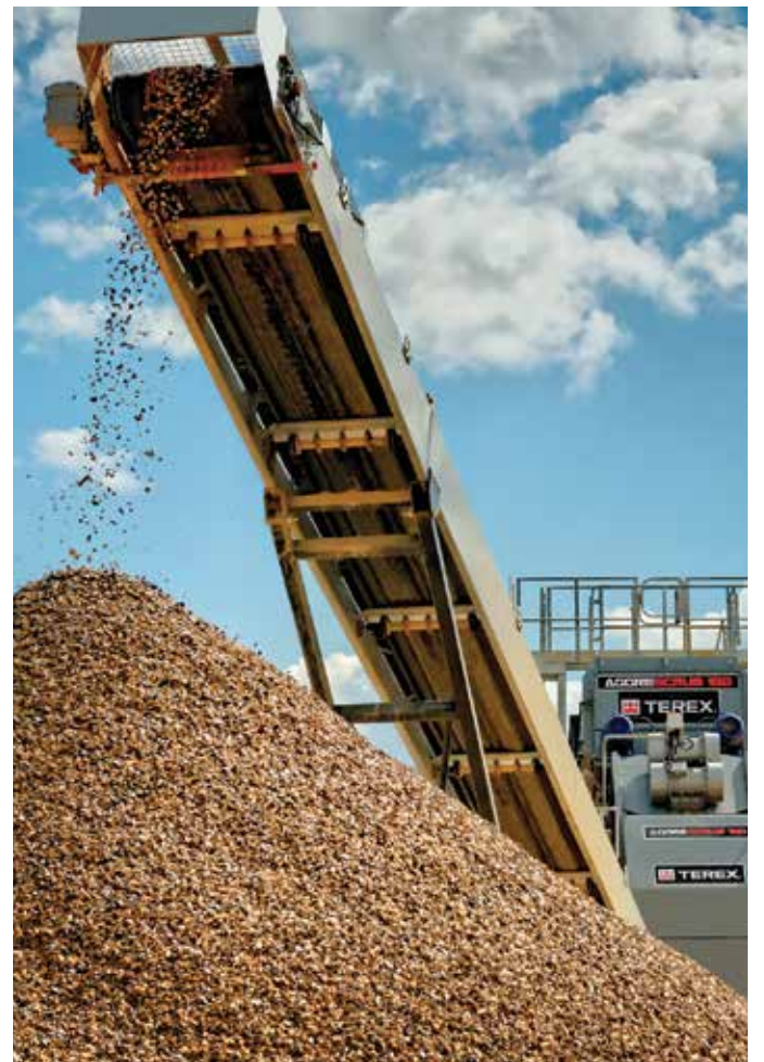
Integral Aggregate Stockpiling Conveyors
