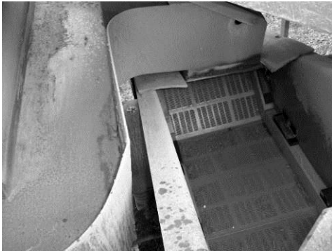
Sloped back panel and modular screen decks
