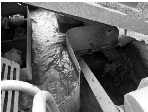
Flume system for transfer from hull to screen
