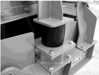
High efficiency rubber screen mount for minimal vibration
