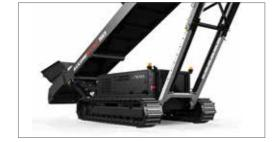
With 400mm dual speed tracks as standard the AggreStac offers speed and control during installation across any
