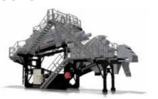
Static and modular systems offering aggressive attrition for sticky and high clay content materials. Highly effective with overburdens, clay-bound ores and recycled materials containing lightweight contaminants.
