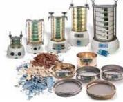
a powerful quality control and acceptance tool. The gradation data is used to calculate relationships between various aggregates or aggregate blends, to predict trends during production and to check compliance with such blends.
