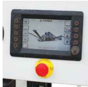
Local machine control panel
