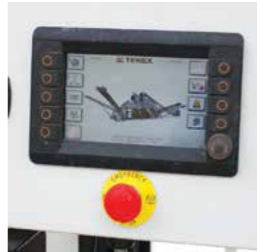
Local machine control panel
