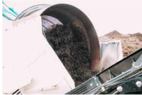
A powerful four-wheel drive system with high performance friction grip wheels is used to turn the trommel drum, giving operators the ability to run it bi-directionally
