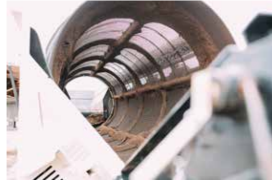
6.45m (21' 2") x 1.94m (6' 4") screening drum with heavy duty mesh or punch plate options offering application flexibility
