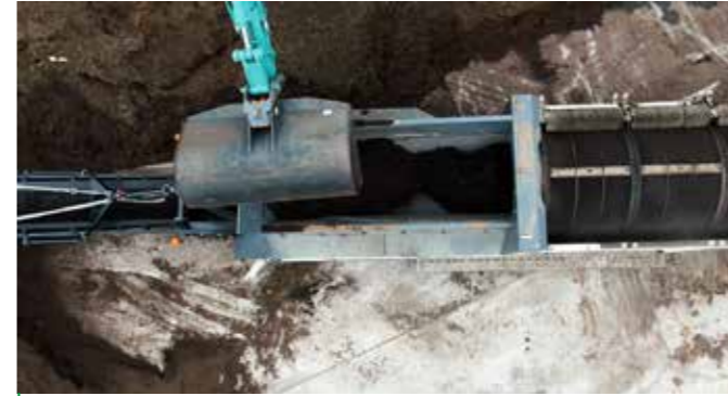
Fully proportional, hydrostatic feeder with an intelligent control system optimising screening performance and throughput
