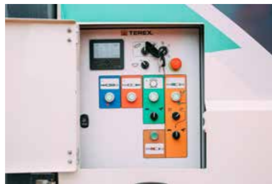
User-friendly push button control system with Auto Start / Stop function and Automatic feeder mode
