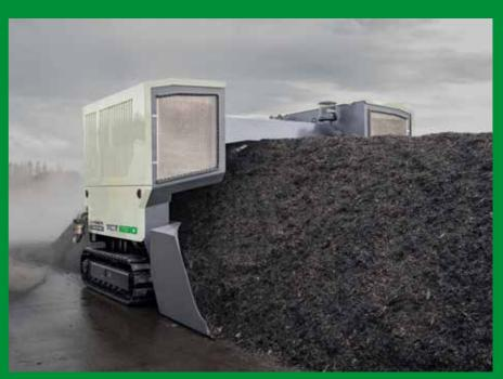
At the core of the TCT 630's design is its latestgeneration rotor, engineered to efficiently lift, aerate, and homogenize windrows while minimizing the shredding of contaminants. This ensures downstream processing remains efficient, preventing complications from overly fragmented impurities.
