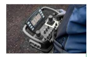
Remote control and semi-autonomous operation enhance operator safety, featuring customizable wear part fields and live turner images. An optional comfort cab is available for extended use.
