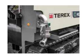
Optional irrigation system balances moisture during composting with easily preset parameters.
