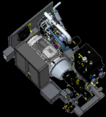
A highly efficient WEG electric motor combined with a hydrostatic drive creates a very responsive shredding action with protection against unshreddable contaminants
