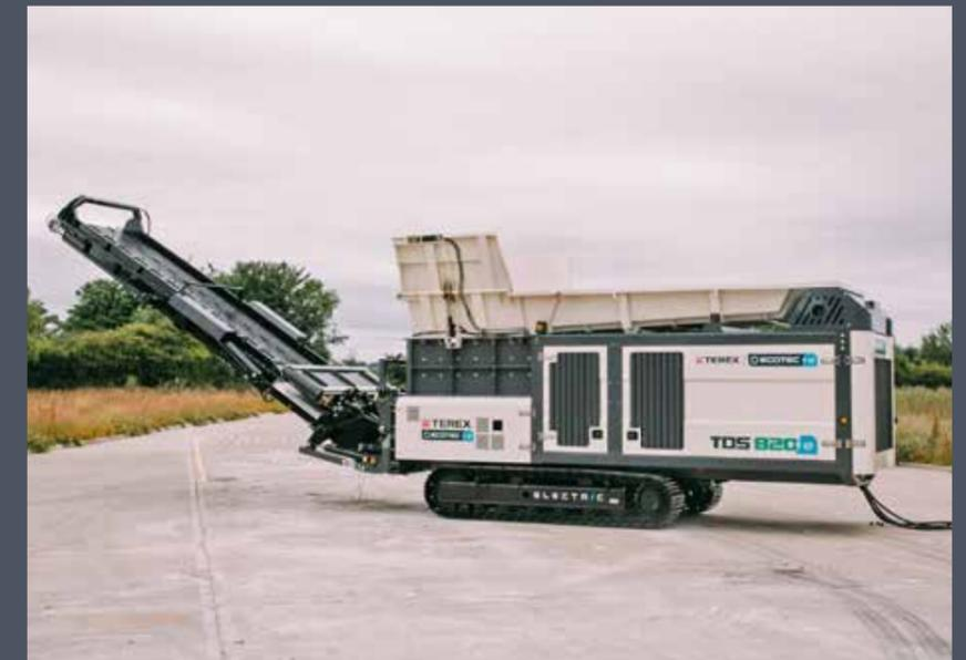
More environmentally friendly in terms of emissions and noise the TDS 820e replaces the Scania DC13 diesel engine with a powerful 280kW WEG electric motor. This change also results in reduced maintenance time and costs. The TDS 820e is fitted with a small 55kW CAT C2.2 engine for tracking and machine set-up, resulting in minimal down time.
