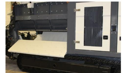
Full chamber access for servicing and breaker bar replacement
