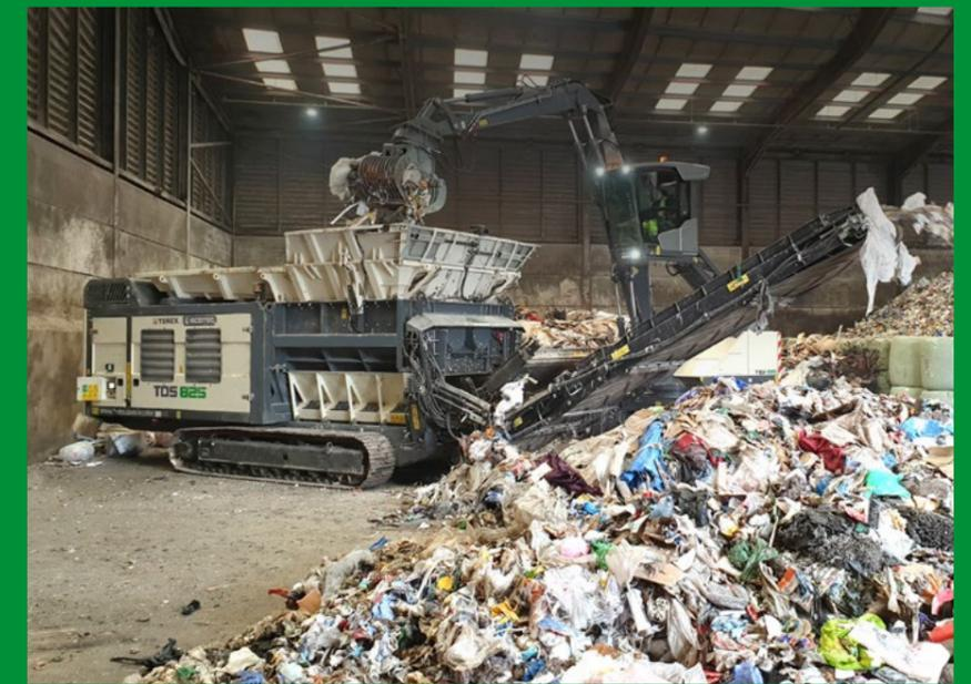
Key features include the hydrostatic drive which offers protection against contamination and allows for bi-directional shredding. The double shaft shredder has 2.5m long shafts made from solid steel, with a fully welded tooth configuration giving an extremely high production rate with excellent size reduction.
