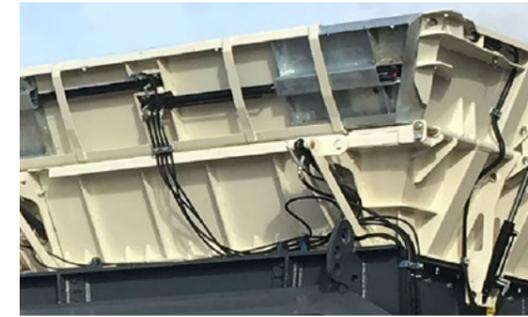
Hydraulic folding hopper extensions allows for increased capacity. Quick and easy set-up from ground level in a matter of minutes (Optional)
